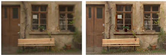
Figure 1.9: To test the capability of our approach to optical aberration correction, we built a camera lens containing a single glass element only. An example image is shown on the left, which exhibits strong blur artifacts especially towards the corners of the image. In contrast, the restored image (right) is of high quality and demonstrates that our method [472] is able to correct for most degradations caused by optical aberrations from a single input image only.
